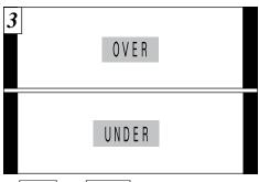
If "OVER" or "UNDER" is displayed, the white balance was not measured at the correct exposure. Reset the white balance.
